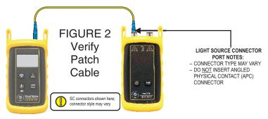
Press 🕖 to power on the Laser OWL singlemode laser source. The 1310nm port powers on first by default.
