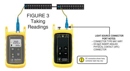
Press 🖀 on the WaveTester to store readings for both 1310nm and 1550nm simultaneously for the current fiber under test.
