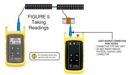
Press 🞬 on the WaveTester to store readings for both 850nm and 1300nm simultaneously for the current fiber under test.
