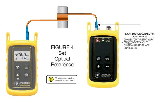
8 Compare the reading on the WaveTester to Table 1 for acceptable power levels. The patch cable should be replaced if it is below the acceptable power level.
