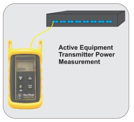
Power on the transmitter port according to manufacturer instructions, if necessary.
