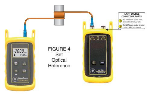
Compare the reading on the WaveTester to Table 2 for acceptable power levels. The patch cable should be replaced if it is below the acceptable power level.
