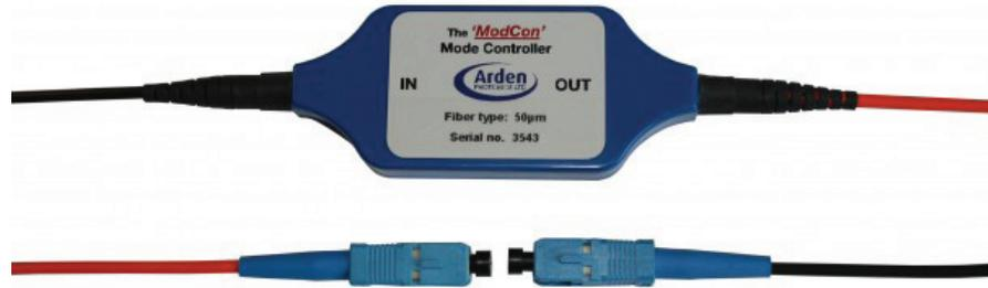
The use of EF-compliant test cables is typically focused on testing OM3/OM4 multimode fiber networks running at 10-gigabit or greater, and usually only when a cabling standard specifies it. Technicians should consult customer documents or applicable cabling standards to verify if EF-compliant testing is required.
