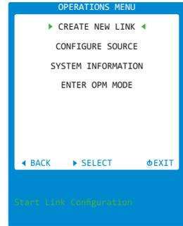
**OPERATIONS MENU > CONFIGURE SOURCE** -- Control the light source port in the MASTER
