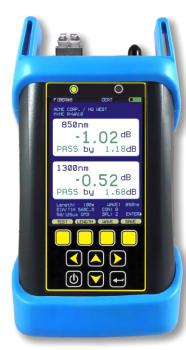
The **Fiber OWL 7V** is a highly accurate hand-held optical power meter, capable of performing a wide range of functions from simple optical power and loss measurements to full-featured standards-based link certification (when used with a WaveSource Pro light source\*) with built-in visual fault location.
