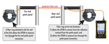
DEAD ZONE BOXES. Dead zone boxes, on the other hand, have adapters installed on the ends of a long spool, and short patch cables are required to make the final connection to the OTDR and the link under test.
